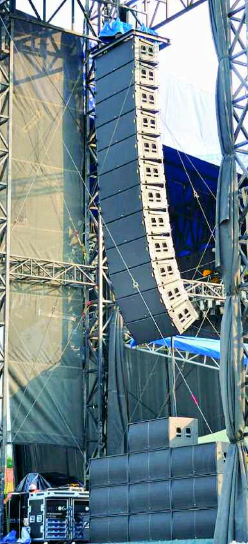
A shot of the Cellular South Stage with the Aero 48 line arrays and the LX-218 subs.
